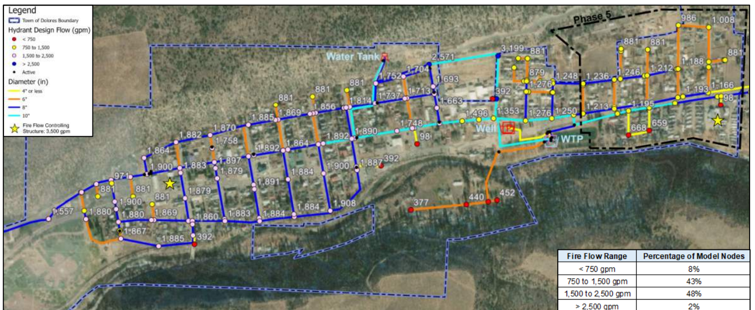
Figure 3-5. Phase 5 Available Fire Flows
