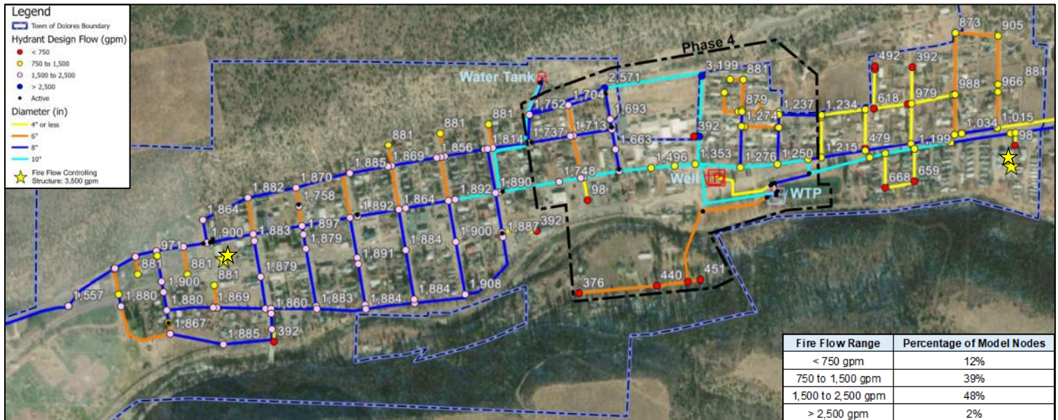
Figure 3-4. Phase 4 Available Fire Flows
